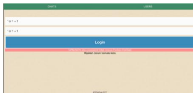
Gambar 9. Pengujian SQL Injection (bypass login)
