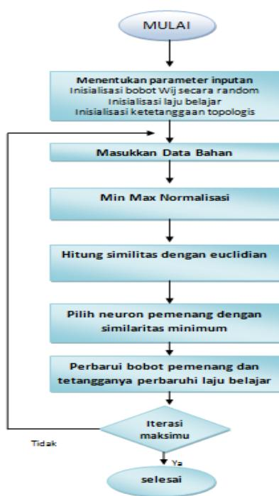
**Gambar 1** flowchart algoritma SOM
